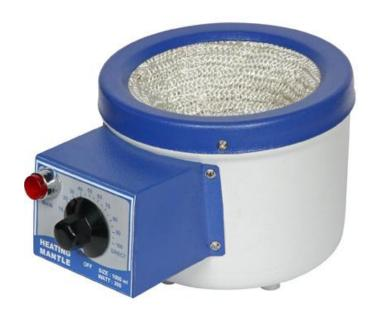
Most suitable for Labs, Pharmaceuticals, Chemicals Glass Plants Etc. Useful for heating inflammable liquids electric heating net is hard Knitted from glass yarn (without any joint) & for durability &stands temp. Up to 350° C body of mantle is spun one piece from non rusting Alum (duly stove 1powder coated) mantles are logged with special grade mineral wool. Most suitable to work on 230 V A.C. supply.
