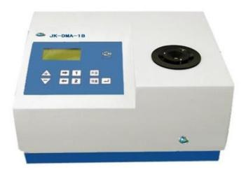
We have various models of Melting Point Apparatus to suit the need of different customers. The Melting point apparatus is designed to determine the melting points with high accuracy, and is supplied with a silicon oil bath with heater for heating the bath. The unit has an arrangement to hold the capillary containing the sample in uniformly heating media.
