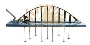
Experiment on a two Hinged arch for horizontal thrust & influences line for horizontal thrust.
