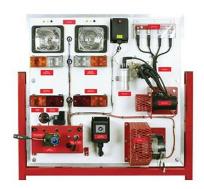
This trainer should be designed to teach students principles of Automotive Electrical System through comprehensive practical activities. The activities include basic of fault finding, battery and fuse, starter and solenoid, relay, horn, turn lights, park lights, license plate light, tail lights, head lamps, direction indicator and hazard light, brake and reverse lights.
