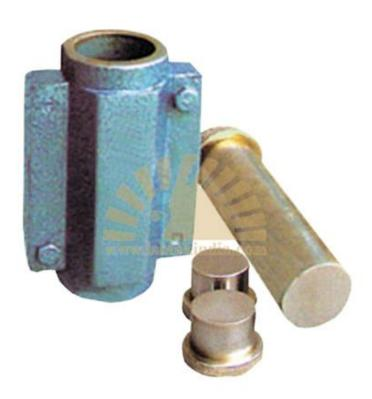
Often in the laboratories it is required to quickly prepare remoulded soil specimen for Triaxial and Unconfined tests. Constants volume moulds are used for this purpose, using either dynamic or static compaction. The moulds are available in different sizes. For specimen size 38 mm dia x 76 mm long comprises. Split mould 38 mm dia x 126 mm long. End plugs 38 mm dia x 25 mm long pair. Split collar interchangeable. Ejecting plunger 38 mm dia x 126 mm long.
