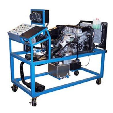
This trainer should be designed to teach students principles of Vehicle Display System and warning systems through comprehensive practical activities. The activities include instrument cluster, fuel system warning system, engine sensor warning system, automotive lighting instrumentation, passenger safety warning system, ABS failure warning system and engine failure warning system.
