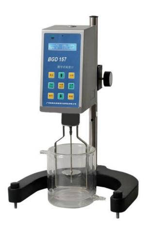
Brookfield instruments use a rotating spindle immersed in the fluid to measure viscosity.
