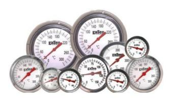
Dial Thermometers are useful for measuring the temperature of Soil, Bitumen or any hot material where inserting glass thermometer is risk from breakage point of view. These are essentially bi-metallic thermometers, bimetal element is enclosed in a hollow metallic stem with close fitting. As the temperature rises bimetal element expands and activates a pointer fixed on the dial to read temperature.
