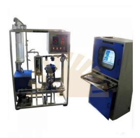
The Level Control System Trainer is the system which outlines the basics of closed loop level control process and other aspects related to it.
