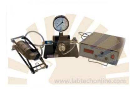
Pressure to Current (P to I) Trainer: This setup comprises of pressure chamber fitted on a base board. A pressure transducer and bourdon pressure gauge are fitted to the chamber. Digital pressure indicator with transmitter output is provided to display the pressure sensor by the pressure transducer. Transmitter output 4 to 20mA can be measured by a current meter. Foot air pump is provided to build the pressure.
