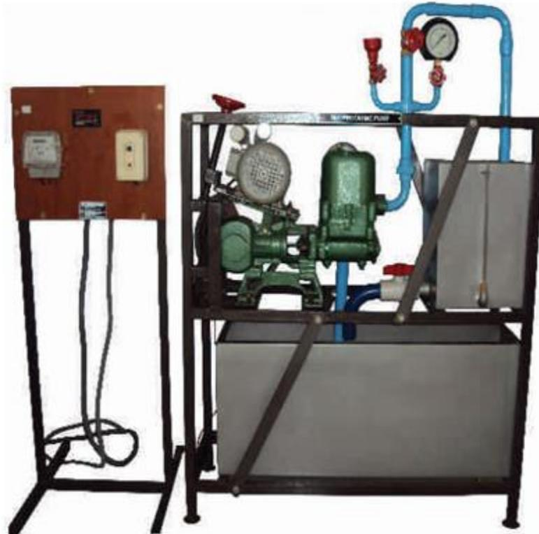
**PRINCIPLE:** Reciprocating pump operates on the principle of pushing of liquid by a piston that executes a reciprocating motion in a closed fitting cylinder.
