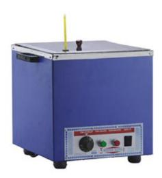
Double walled inner chamber in stainless steel outer chamber in mild steel temperature range Ambient to 100° C controlled by capillary thermostat. Accuracy  $\pm$  1° C operated on 230V A.C. Single Phase. These baths are suitable for washing Marshall specimen. Lid is made up of stainless steel with a hole for glass thermometer to penetrate.
