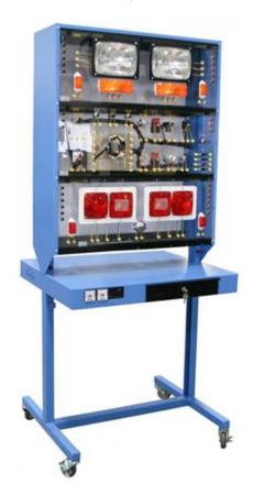
This trainer should be designed to teach students principles of lighting circuits used in modern vehicles through comprehensive practical activities. The activities include interior light circuits, brake (stop) circuit, reverse (backup) circuit, Hi/Lo beam circuit, hazard warning circuit, turn signal circuit, park and tail circuit, relay circuit, vanity light circuit.
