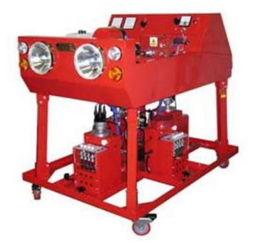
This trainer should be designed to teach students principles of Engine Management used in modern vehicle through comprehensive practical activities. The activities include fundamentals of fuel system electronics, transducers, Engine Control Unit, actuators, emission control, self diagnosis and trouble codes.
