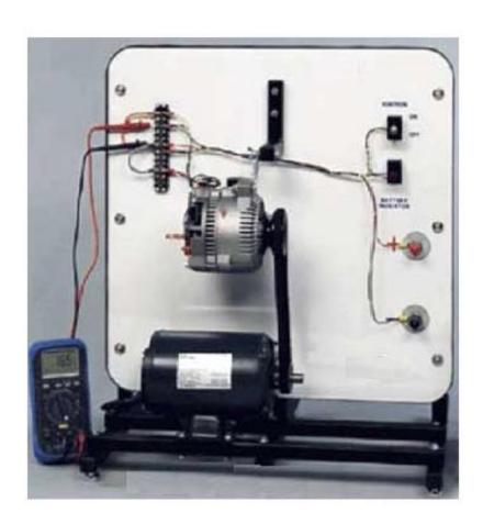
This trainer should be designed to teach students principles of Ignition system used in modern vehicle through comprehensive practical activities. The activities include semiconductor familiarization, transistor basic circuit, contact breaker ignition, wasted sparked ignition, electronic ignition systems, spark plugs, and alternator charging systems.
