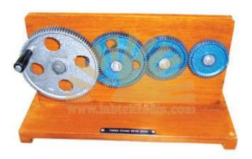
Gears are employed as a link between drive machine and work machine. They are used to vary torque and speed and to change direction. The aim of dynamic gear analysis is an understanding of the motion sequences and the influence of inertia.
